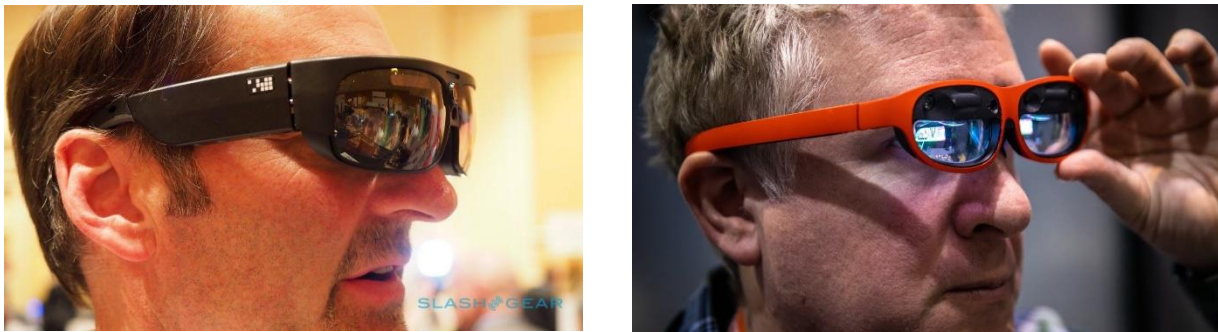
Fig 1: Two curved mirror display based smart glasses (ODG on left and NReal on right).
