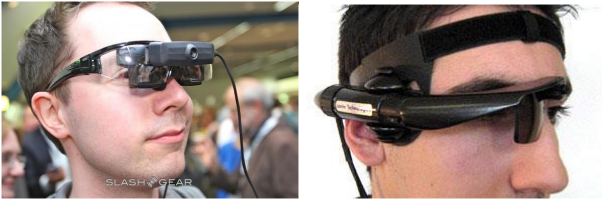
Fig 1: Two curved mirror based wearable AR display technologies (Vuzix on left and Laster on right).
