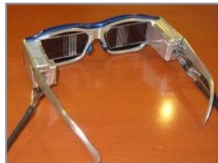
The rear side of the prototype. The saw-toothed lens is needed to superimpose images on the actual sight. Normal sunglass lenses are attached to the front side of the HMD for design's sake. And the aluminum frame of the prototype will be replaced by a light plastic frame when it is commercialized.
